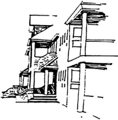
The building form of post and beam is appropriate in a forested environment.
